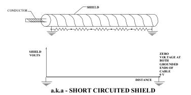
With the shield grounded at both ends over a normal distance, no standing voltage appears. However, assuming a good earth ground path, this configuration is subject to circulating current as it replicates a trans-
